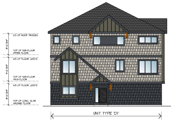
8 BUILDING #2 EAST ELEVATION SCALE : 3/16" = 1'-0"
