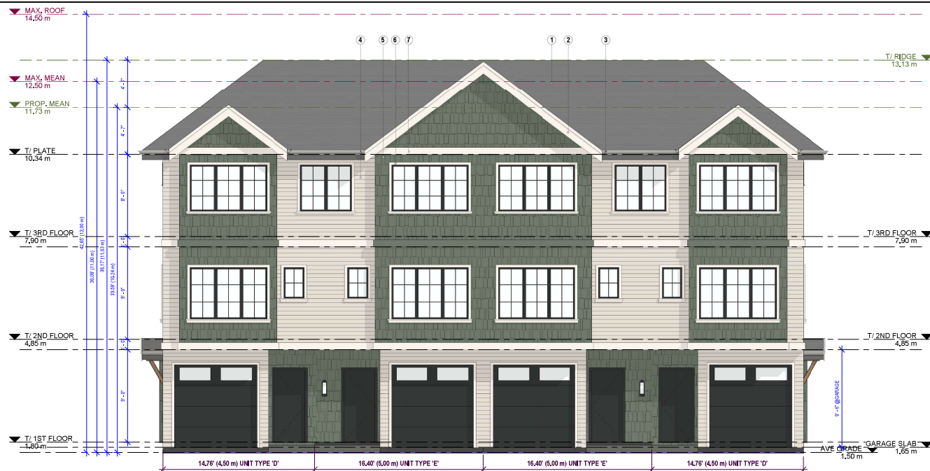
BUILDING 3 - FRONT / NORTH ELEVATION
