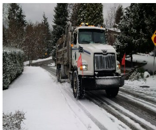
9 -Tandem axle dump trucks with Sander and belly plows (4 of which also have front mount plows).
