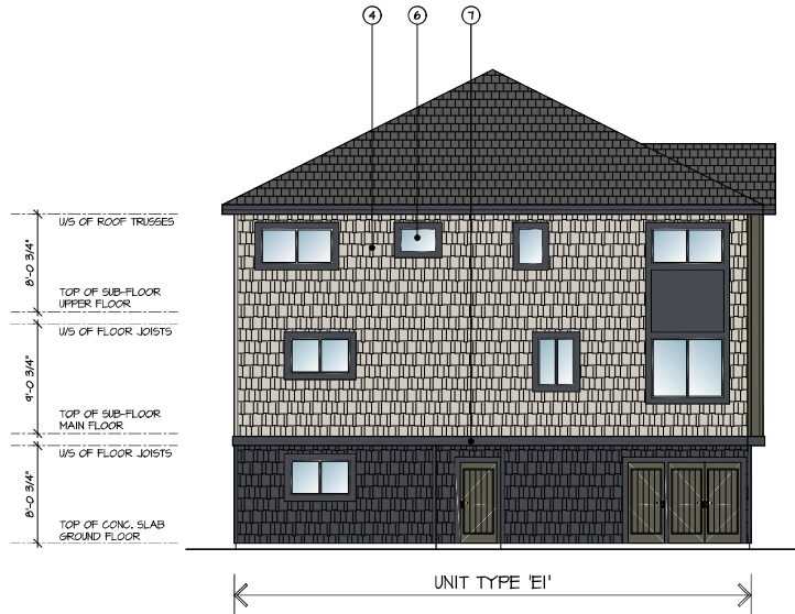
3 BUILDING #1 WEST ELEVATION SCALE : 3/16" = 1'-0"
