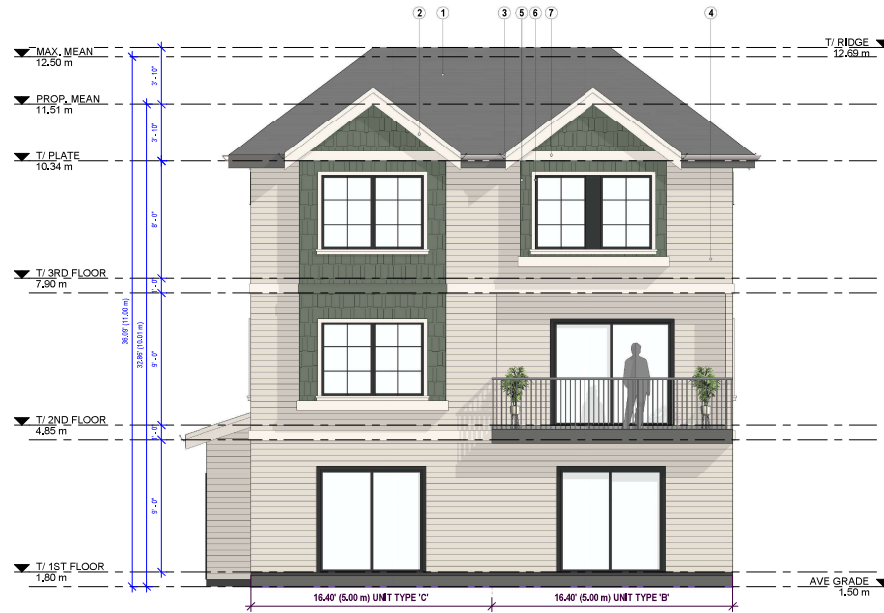
BUILDING 2 - REAR / EAST ELEVATION
